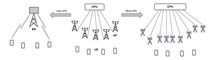
Fig. 1. The unified model for cellular/cell-free massive MIMO, where M antennas are distributed over  $N_{AP}$  APs. If  $N_{AP} = 1$ , it stands for cellular massive MIMO relying on a single base station, as the leftmost diagram shows, while typical cell-free massive MIMO with  $N_{AP} = M$  distributed single-antenna APs is shown in the rightmost diagram.
