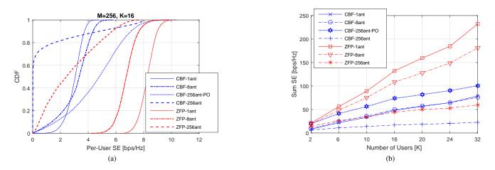
Fig. 2. Performance comparison in the downlink of massive MIMO systems: (a) the CDF curves in terms of per-user SE using ZFP and CBF, where M = 256 antennas serve K = 16 users; and (b) the achievable sum SE in terms of the number of users when M = 256.
