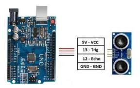
Figure 2. Connection diagram
